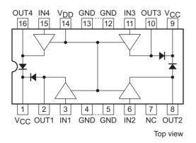
Note: V<sub>CC</sub> (pins 1 and 9) is shorted internally.
